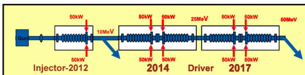
Figure 1: Conceptual layout of the TRIUMF e-Linac.
