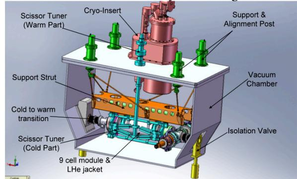
Figure 5: The injector cryomodule for e-Linac.
