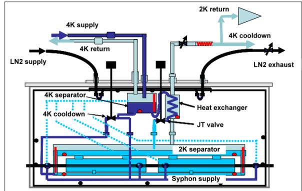
Figure 4: Cryomodule cryogenic circuit showing cold mass, 4K phase separator, 4K cooldown circuit, JT valve and heat exchanger. The dashed line indicates the siphon return circuits from 4K intercepts.
