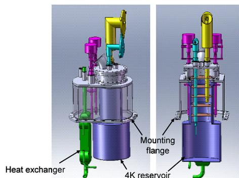
Figure 6: The 4K/2K cryo-insert for the ICM and ACM.
