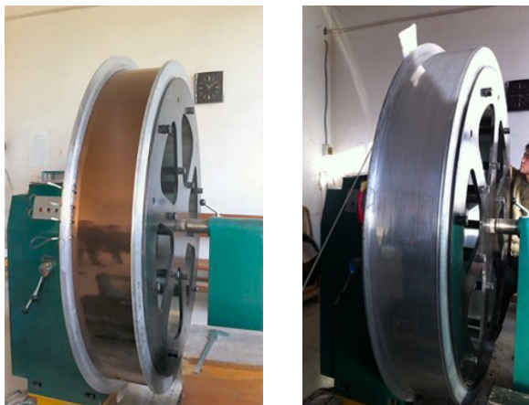
Figure 5: The left photo shows the superconductor winding complete. The right photo shows the aluminum banding wound over the superconductor.
