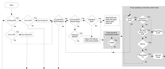
Figure 5: Pump logic diagram.
