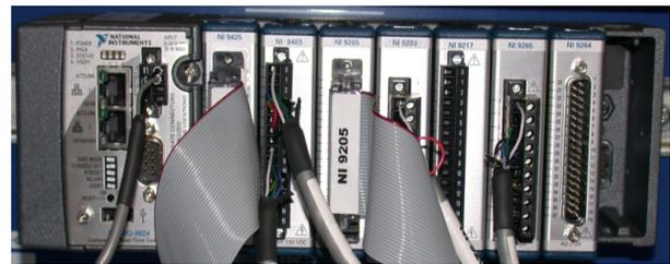
Figure 3: NI cRIO with I/O modules installed.
