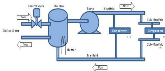
Figure 1: Drift tube linac water cooling system.
