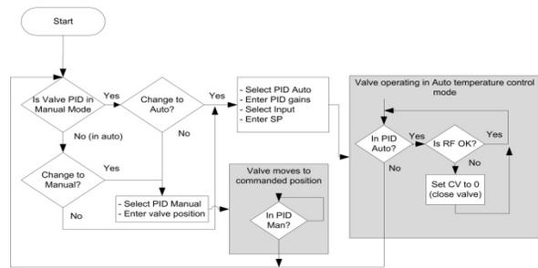
Figure 6: Valve logic diagram.
