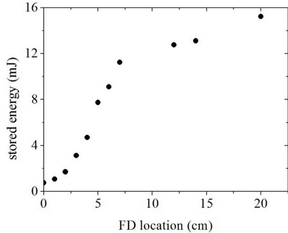
Figure 5: Stored energy in the cavity versus various locations of the FD during extraction, with 23kHz of detuning from the tuning plate.
