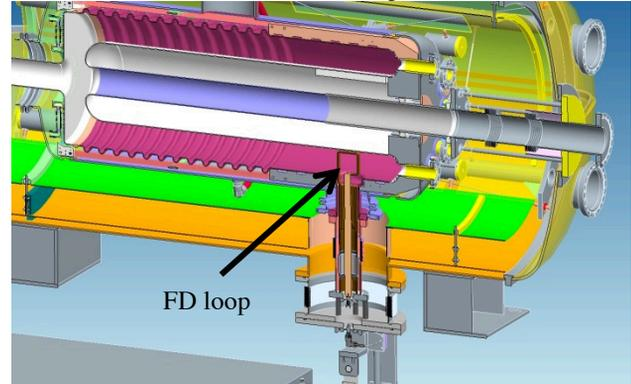
Figure 1: Cross section of 56MHz cavity with the Fundamental Damper fully inserted.
