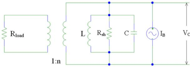
Figure 3: Circuit diagram representing the 56MHz cavity with the FD inserted.
