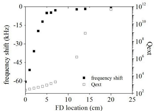
Figure 2: 1. Solid squares: Frequency shift versus the various insertion locations of the FD. 2. Open squares: External Q of the FD port versus the various insertion locations of the FD.
