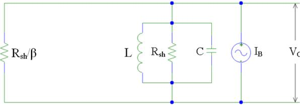
Figure 4: Simplified circuit diagram representing the cavity with the FD inserted.
