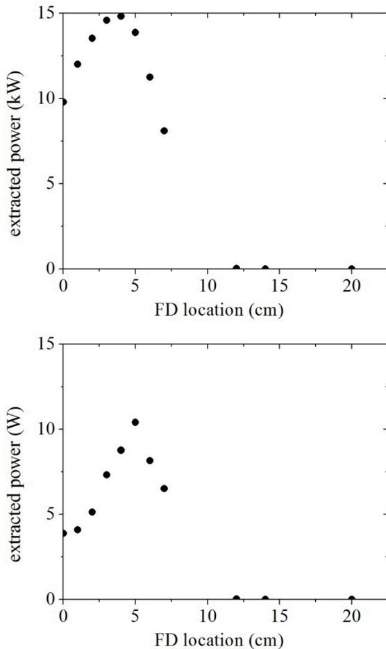
Figure 6: Upper: Extracted power to the external load of the FD system versus various locations of the FD. Top: Only 23kHz detuning from the tuning plate; Bottom: Both 23kHz detuning and the frequency shift due to the FD.
