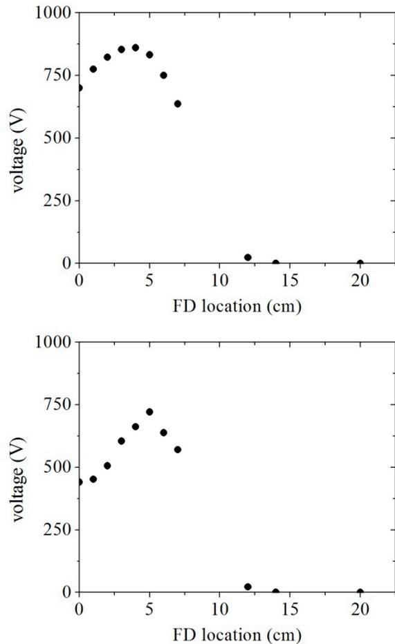
Figure 7: Voltage across the inner and the outer conductor of the FD plotted against various FD locations. Top: Only 23kHz detuning from the tuning plate. Bottom: Both 23kHz detuning and the frequency shift due to the FD.
