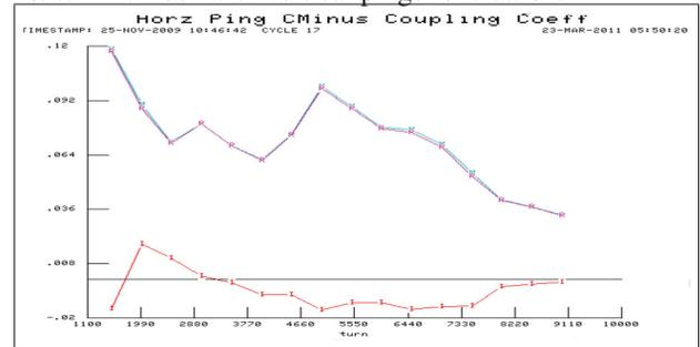
Figure 3:  $\mathcal{R}(C^-)$  (green),  $\mathcal{I}(C^-)$  (cyan) and  $|C^-|$  (red) vs. turn number with horizontal pinger excitation.
