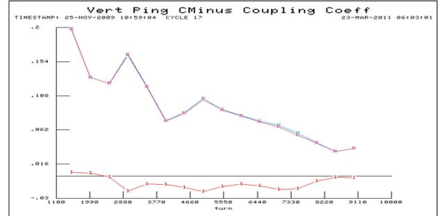
Figure 2:  $\mathcal{R}(C^-)$  (green),  $\mathcal{I}(C^-)$  (cyan) and  $|C^-|$  (red) vs. turn number with vertical pinger excitation.
