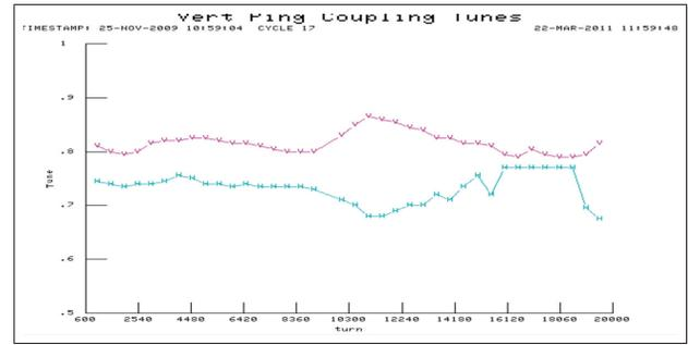
Figure 1: Horizontal (red) and vertical (green) tune vs. turn number with vertical ping excitation.
