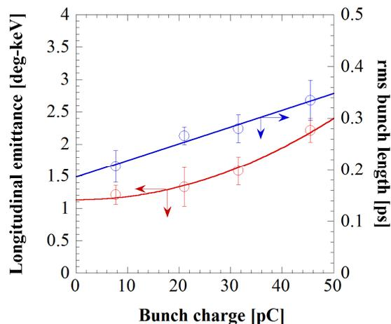
Figure 3: The longitudinal emittance and bunch length as a function of bunch charge.
