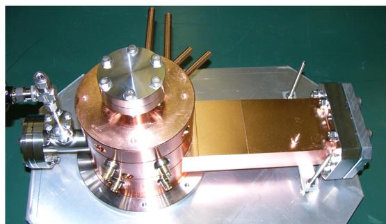
Figure 1: The structure of the rf cavity and the picture of the completed rf gun.
