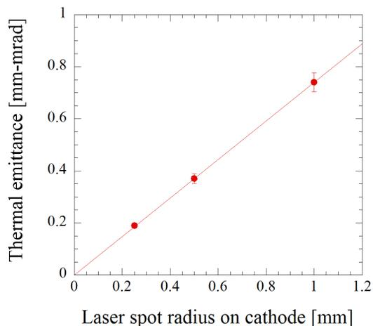
Figure 2: The thermal emittance as a function of laser spot radius on the cathode.
