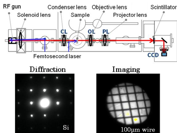
Figure 4: RF gun based MeV UED system, the electron diffraction and imaging obtained by 3 MeV electron beam.
