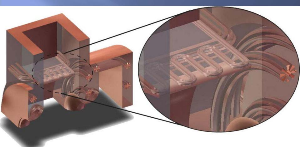
• Six conformal channels and four snake-like around the coupling iris regions with starshaped cross-sections
