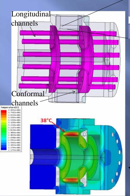
Coupling window Cooling channel
