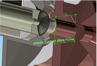
~20% current loss between emitter and anode slice plane – additional diagnostics required.
