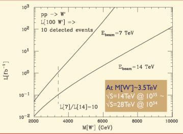
However, energy upgrade is extremely difficult from the accelerator standpoint Many issues, but key R&D challenge is developing the high field dipoles
