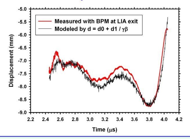
This sweep is unlikely the result of the resistive-wall instability growth, which is independent of energy in a solenoidal focusing field.
