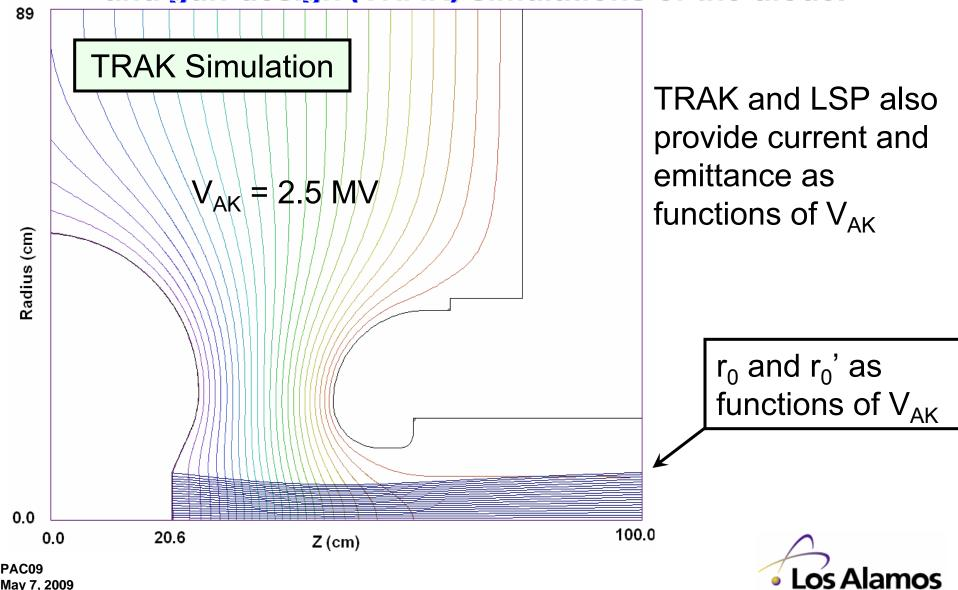
Initial conditions as functions of diode voltage from simulations were converted to initial conditions as functions of time using measured diode waveforms.
