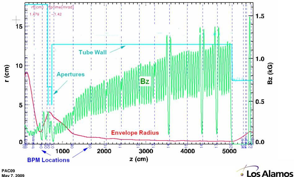
The 2-kA electron beam is transported through the accelerator without losses.
