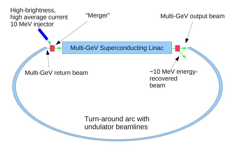
Energy recovery addresses the most significant advantage of rings over linacs.
