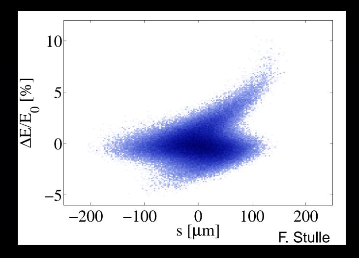
Negligible longitudinal phase space deformation in the RTML at 8 GeV. THEFF047
