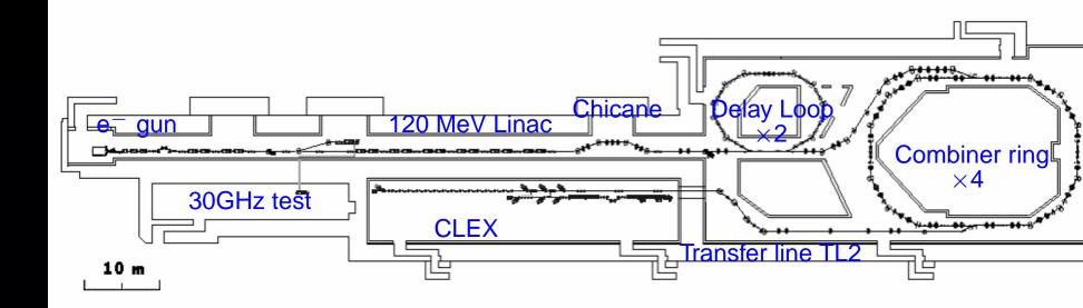
CLEX is where the high intensity beam (drive beam) transfers its energy to the main beam.
