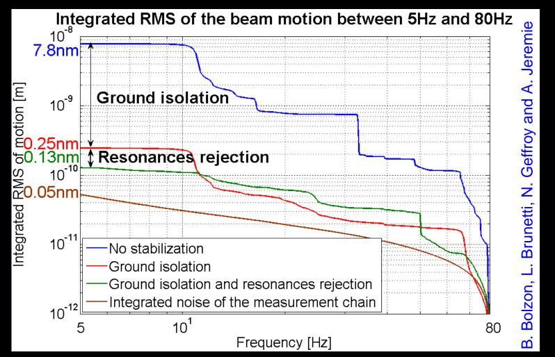
0.13 nm reached in laboratory, the challenge remains to prove 0.15 nm within the detector.
