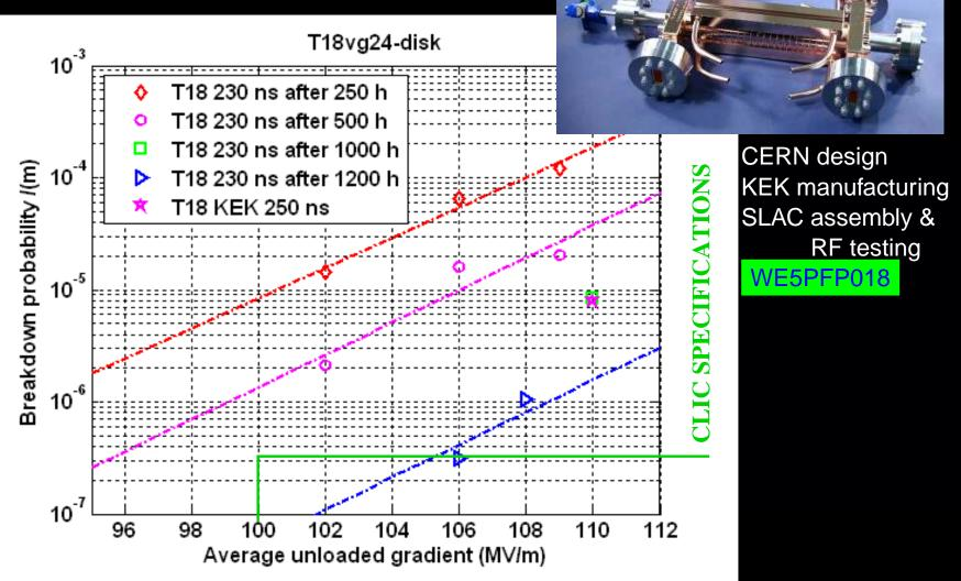
Demonstration of CLIC specifications with a CLIC-like structure without damping.
