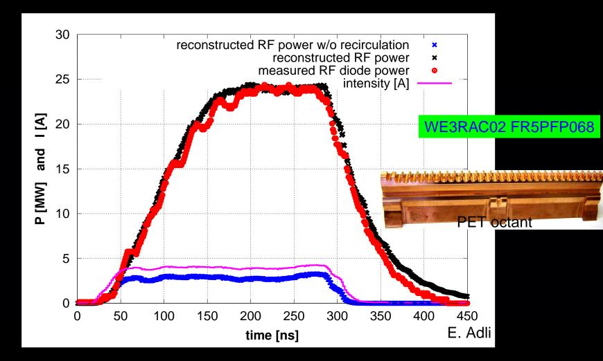
Power extraction demonstrated @ 3 A. Enhancement by power recirculation in the PETS.
