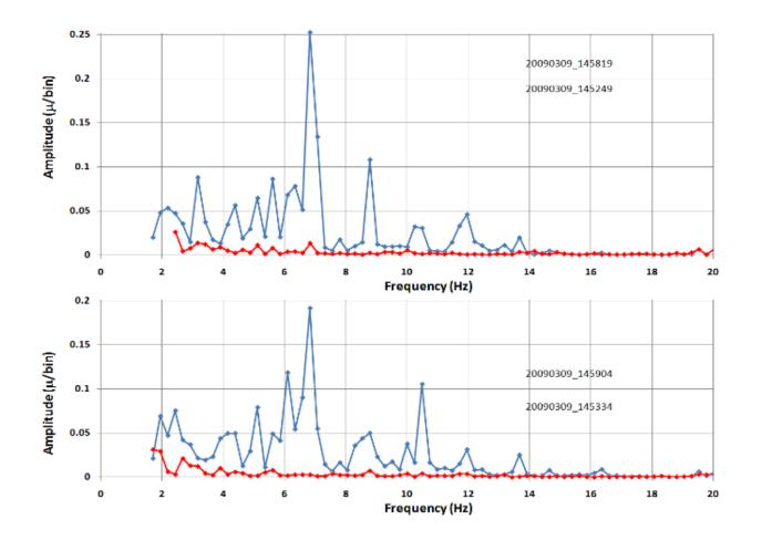
Vibration spectra of one triplet cold mass, with and without active damping
