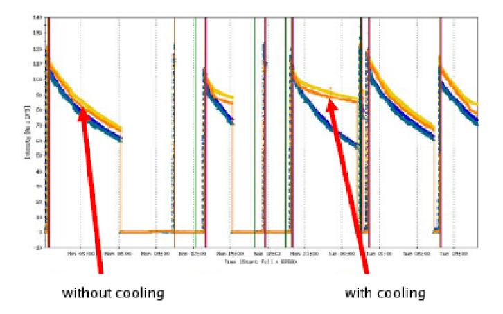
IBS leads to debunching; debunched particles continuously removed from abort kicker gap Image courtesy of Mike Brennan
