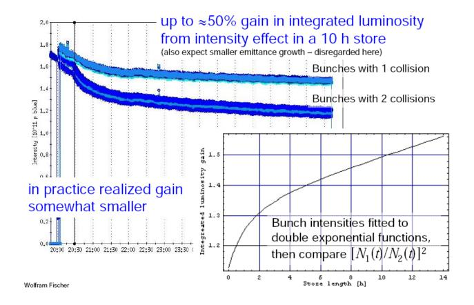
Proton beam lifetime is limited by beam-beam effect; bunches with one collision have longer lifetime than bunches with two.
