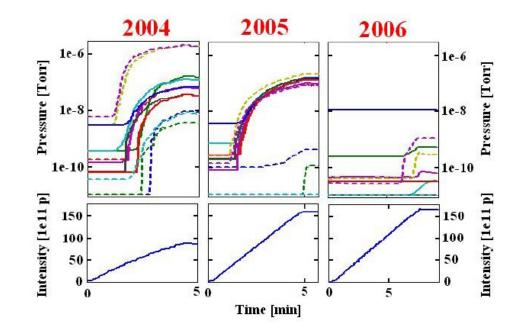
Dynamic pressure rise during beam injection, caused by electron clouds Vacuum system upgrades:
