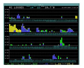
Figure 4: Logarithmic display of losses around the Main Injector. Integrated loss at the end of the cycle are displayed in green. Losses after the uncaptured beam loss overlay this in yellow. Losses at the end of injection overlay this in blue. Various sums and intensities are displayed at the top and bottom. For this display, the collimation region includes 229 - 309.
