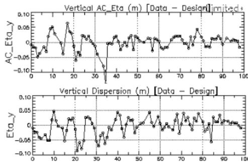
Figure 3: Top: New AC dispersion measurement. Bottom: Standard dispersion measurement.
