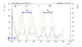
Figure 1: Original half FF optics. The IP is located at 0.0 meter followed by the vertical  $(-I_y)$  and horizontal  $(-I_x)$  chromaticity correction section. The crab waist sextupoles are located on the far right hand side.
