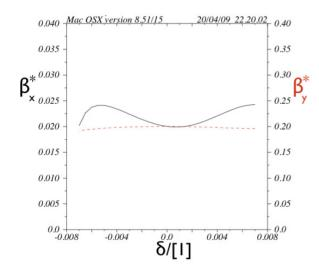
Figure 7: Bandwidth plot. The black curve depicts the horizontal, the red the vertical IP  $\beta$ -function as a function of the energy.  $7 \times 10^{-3}$  corresponds to ten times the energy spread of the beam.
