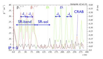
Figure 5: TWISS functions of the new right half of the FF.
