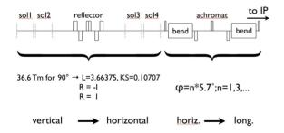
Figure 3: Standard arrangement of an spin rotator using solenoids and horizontal dipoles.
