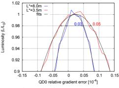
Figure 8: Relative luminosity versus relative QD0 gradient error for the two L\* options.
