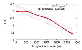
Figure 1: The CLIC BDS layout with parallel lines showing the direction of the beam at the IP. The polarimeter should be placed in a location parallel to the IP.
