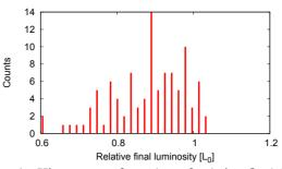
Figure 4: Histograms of number of relative final luminosities after a maximum of 18000 tuning iterations of the CLIC FFS. 80% of the seeds reach 80% of the luminosity with a prealignmenet tolerance of  $10\mu$ m.
