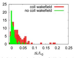
Figure 2: Relative luminosity loss of 100 simulated machines, assuming  $0.2\sigma_y$  jitter at the BDS entrance without any feedback. The vertical collimator gaps are set to  $44\sigma_y$  (as shown later the new depth is  $55\sigma_y$ ).
