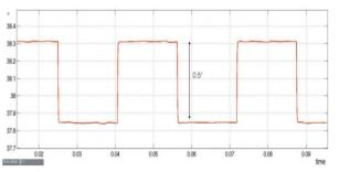
Figure 5: Stabilized cavity phase for 23 Hz square wave detuning and loop gain of 120
