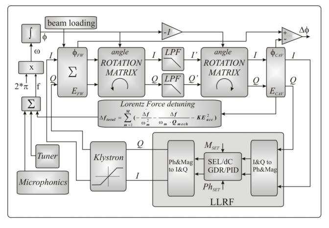
Figure 1: Diagram of the RF System model
