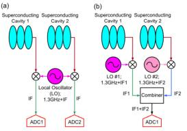
Figure 1: Schematic diagram of the digital LLRF system: (a) Typical system and (b) IF-mixture technique.
