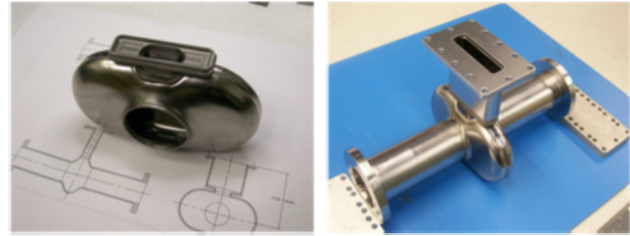
Figure 3: Second niobium prototype of on-cell waveguide coupling to cavity cell, left: after the first EB-weld, right: stack assembly before the final EB-weld.
