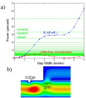
Figure 2: a) Coupling ratio as a function of gap length and the reflection amplitude to be matched by a ridge; b) Half cross-section with electric field plot for a 7.9375 cm gap, tapping off about 6.6% or 1/15 of the power.
