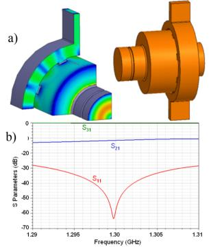
Figure 3: a) Quarter geometry of a CTO design with field patterns (magnetic on outer cylinder) and full model; b) Simulation S matrix plots showing an excellent match and a -11.63 dB coupling.
