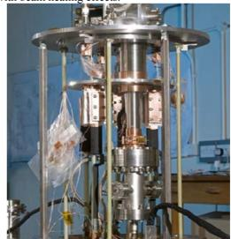
Figure 6: The cryostat turret.
