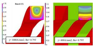
Figure 2: The peak field in conductor with and without no iron present, to deliver same bore field Bo.
