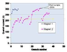
Figure 7: Results from the critical current testing of the magnets prior to integration in final vessel. Note the yellow line is the nominal current required by the ILC.
