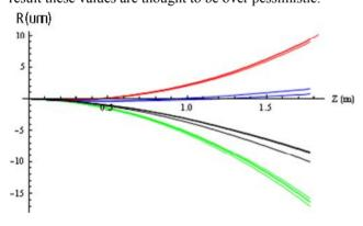
Figure 8: Calculated electron beam drift along magnet 2 the 4 different colours for equally spaced points (90°) around the azimuth, calculated from measured field profiles, using SPECTRA. The same colour calculated for same field orientation measured with different hall probes.
