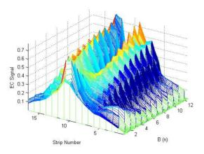
Figure 6: Electron signal vs. strip collector number vs. n for aluminum surface showing increases in density due to resonances.
