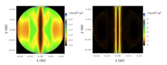
Figure 2: Density distribution for a resonant (0.07T) and non-resonant (0.08T) case. Vacuum chamber is circular and fits exactly within the plot.
