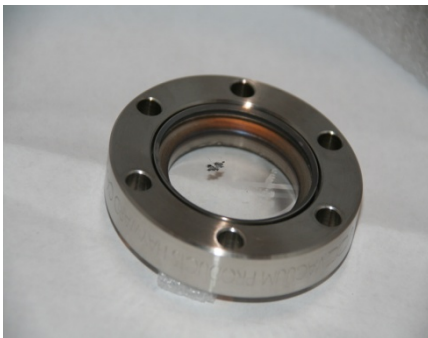
Figure 3: Vacuum window which limited the laser power to the H^- beam in the experiment described above.
