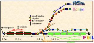
Figure 1: Schematic layout of the SPARC and related experiment area. The part dedicated to Plasmon-X and Thomson can be used to experimentally verify the calculations of this work
