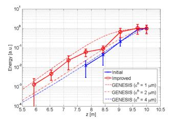
Figure 1: Experimental energy gain curves before (solid blue) and after (solid red) optimization of SASE FEL. Saturation is observed at 9-m in the 10-m long NISUS undulator. GENESIS results are shown as the dashed and dash-dotted lines in red and blue with different normalized emittances, charges, and bunch lengths.
