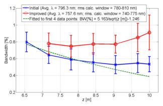
Figure 2: Experimental evolution curve of the spectral bandwidth along NISUS before (blue) and red (after) optimization of SASE. The bandwidth is narrower and decreasing in the barely saturated case, but broader and increasing in the case of deep saturation.
