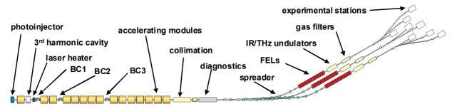
Figure 1: Schematic layout of the NLS facility.
