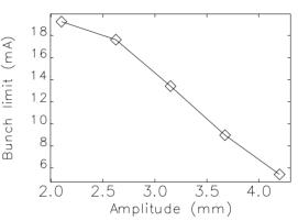
Figure 2: Bunch charge limit as a function of imparted horizontal betatron oscillation.
