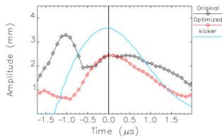
Figure 3: Betatron oscillations on non-targeted bunches as a function of time about the targeted bunch for two sets of sextupole settings. Ideal kicker waveform is superimposed.
