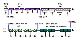
Figure 1: Layout of LINAC RF modules.
