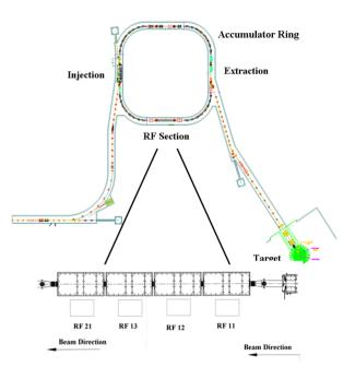
Figure 2: Layout of ring RF components.
