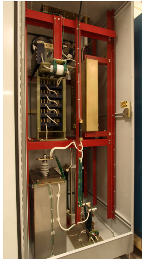
Figure 4: High-voltage cabinet for the pulsed amplifier. The modulator is at the middle left, and has blue switch plates. This cabinet is air-insulated.
