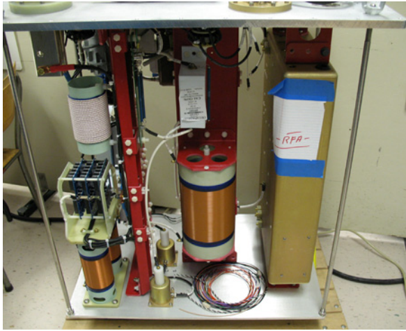
Figure 2: Tank for the CW amplifier. This tank holds the high-voltage power supply, and auxiliary floating supplies. The tank is insulated with oil.
