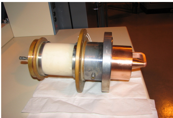
Figure 1: Photo of cavity input coupler.
