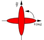
Figure 2: Bunch compression by fast bunch rotation. The primarily bunch in the horizontal position will be rotated by 90° into an upright position.
