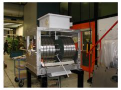
Figure 3: The bunch compressor cavity loaded by 20 MAring-cores (VitroVAC 6030F). The box on top of the cavity contains the adjustable gap capacitors to tune the cavity.
