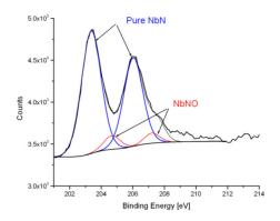
Figure 4: XPS measurements of NbN coupons.
