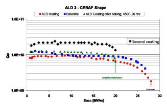
Figure 2: High temperature baking on ALD coated cavity#1. In bleu the ALD baseline, in red the RF test after the 450C-20hrs baking, in pink after the first HPR and in green after the second HPR.
