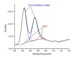
Figure 3: XPS spectrum of ALD made Niobium metal.
