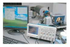
Figure 4: Photograph of the RadiaBeam Terahertz laboratory setup where the interferometer and detector are being tested with a calibrated blackbody source and a 10.6  $\mu$ m CO<sub>2</sub> laser. The results are compared to the standard Michelson scanning interferometer.
