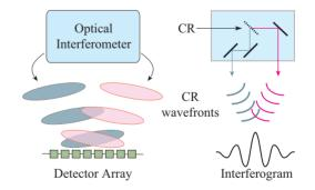
Figure 1: Conceptual scheme of the real-time interferometer which autocorrelates the phase fronts of beam-based radiation to determine bunch length information.
