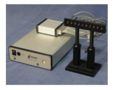
Figure 3: Example of a 10 channel joulemeter fabricated by Spectrum Detectors including DAQ and controller. The segmented detector for the real-time terahertz interferometer requires significant enhancements in size and sensitivity.
