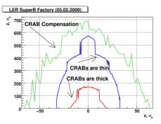
Figure 4: DA aperture due to the kick (blue) and finite length (red) Crab sextupoles and that recovered by the correction sextupoles (green).
