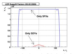
Figure 2: DA reduction due to the finite length of the IR chromatic sextupoles.
