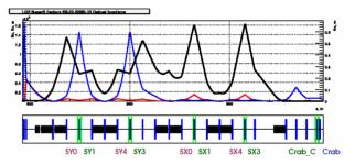
Figure 1: Lattice functions and sextupole arrangement of the LER interaction region (the IP at the left side is the reflection symmetry point of the plot).
