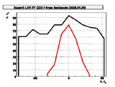
Figure 8: DA reduction due to the sextupole component in the quadrupole fringe field.
