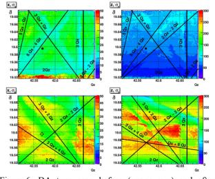
Figure 6: DA tune scan before (upper row) and after (lower row) correction. The color indicates the maximum DA size.
