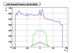
Figure 3: Finite length sextupoles DA (black) and its recover by correction octupoles (green) and sextupoles (blue).
