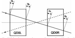
Figure 7: With the crossing angle at the IP the beam passes the quadrupole entrance and exit at some angle.
