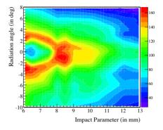
Figure 4: 2D scan of the horizontal polarisation component intensity (in mV) of the CDR spatial distribution
