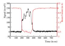
Figure 3: Example CDR signal with corresponding beam current reading from a nearby BPM
