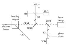
Figure 6: Upgraded CDR setup in the CRM line. A Michelson interferometer, consisting of a beam splitter S1, a fixed and movable mirror, M1 and M2, and a Schottky barrier diode (SBD) detector is installed. Along the OTR optical line a beam splitter S2 is installed, providing a simultaneous beam position and charge reading with the CCD camera and photo diode, respectively.
