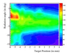
Figure 5: 2D scan of the horizontal polarisation component intensity (in mV) of CSR spatial distribution.
