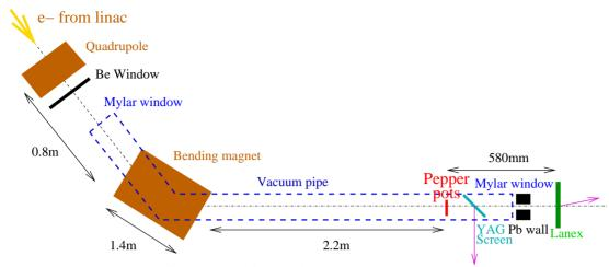
Figure 2: Experimental layout at the DAFNE BTF.
