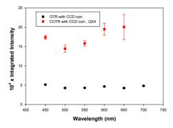
Figure 2: Evaluation of the OTR/COTR image intensities versus the bandpass filter center wavelength for the PC rf gun beam (red) and TC rf gun beam (black). The COTR has a stronger red component than the incoherent OTR.
