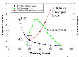
Figure 5: Analytical representations of the OTR dependence on  $1/\lambda^2$  and OTR times the 3-keV gain factor, or COTR. The CCD camera response is also shown.
