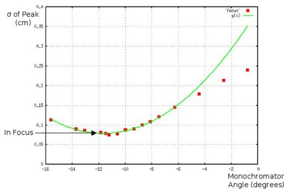
Figure 3: Extracted widths of the 13 image peaks, plotted versus the monochromator setting.
