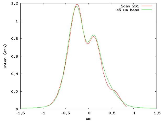
Figure 5: Beam profiles with the Coded Aperture in place under slightly degraded beam conditions
