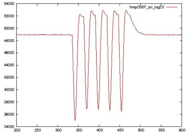
Figure 1: Signal response of our photodiode array. The peak-to-peak temporal spacing is 14 ns corresponding to standard CESR positron bunch spacing. Five CESR bunches are seen in this figure. The 1.5ns rise time seen in the plot is consistent with the preamplifier bandwidth and the S/N evident in these data is characteristic of 100-turn averages.
