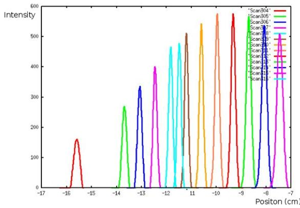
Figure 2: Intensity profiles taken with the FZP at different x-ray energies.
