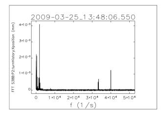
Figure 2: Spectrum of beam horizontal motion from 1 Hz to 50 kHz.
