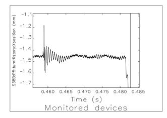
Figure 4: Turn-by-turn record of beam horizontal position preceding a beam dump.
