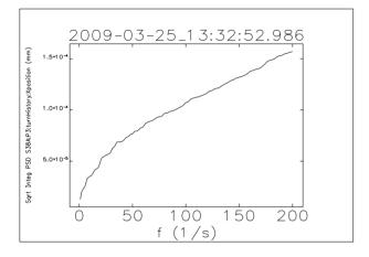
Figure 3: Full system (Buttons to FPGA) noise floor.
