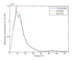
Figure 5: Energy distribution in the baseline run, with primary angular distributions matched.
