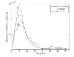
Figure 4: Energy distribution in the baseline run: no SEY, reflectivity, or space charge.
