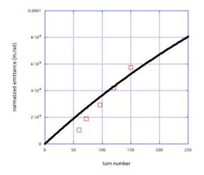
Figure 5: Emittance growth in the vertical direction as a function of turn numbers. Vertical axis in this figure shows a normalized emittance. Open squares show the experimental results and a solid line shows the theoretical estimation based on the ionization cooling model.
