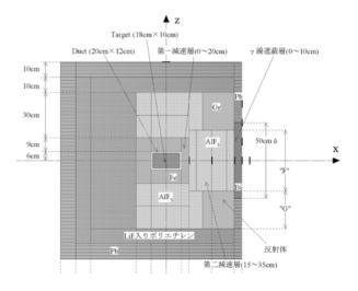
Figure 3: Schematic configuration of neutron moderator.
