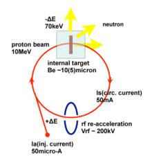
Figure 1: Schematic diagram of FFAG-ERIT.
