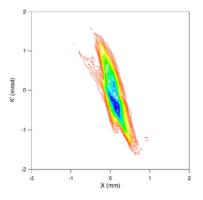
Figure 7: Reconstructed transverse phase space, represented as a contour plot, from the FEL Upgrade driver.
