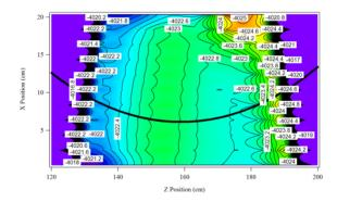
Figure 6: Measured data of a dipole before installation in the Upgrade driver exhibiting 1 part in 10,000 field homogeneity at 145 MeV. The thick black trace represents the beam trajectory.
