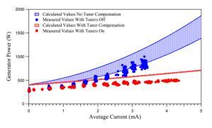
Figure 5: Measured data showing generator power as a function of beam current with the cavity tuners on to compensate for the reactive power (red) and off (blue).
