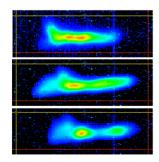
Figure 4: Images from a synchrotron light monitor showing beam filamentation as a function of bunch length compression (courtesy P. Evtunshenko).
