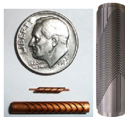
Figure 5: Left; Miniature DDH coil for medical applications. Right: Larger quadrupole coil with an aperture of 100 mm.
