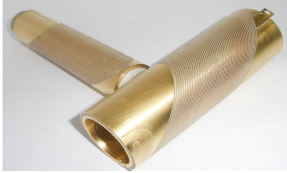
Figure 6: Two sets of DDH coils that fit into each other forming one unit for horizontal and vertical beam steering.
