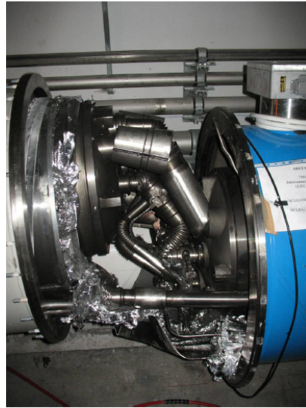
Figure 6: A damage interconnect between a quadrupole and a dipole.
