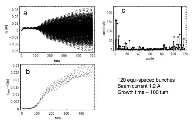
Figure 2: Beam signal (a), beam envelope (b), and mode spectrum (c) for a completely filled DAFNE bunch train.
