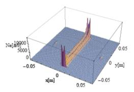
Figure 1: Typical electron cloud distribution in the transverse x-y plane. The number of electrons in an arbitrary unit is plotted in the vertical axis, as obtained by PEI-M after the first bunch train passage in a DAFNE arc bend.
