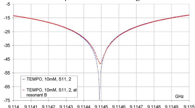
Figure 4: Network analyzer measurement of solid TEMPO (10mM).  $S_{11}$  (reflection) at resonant magnetic field ( $h\nu = g_e \mu_b B_0$ ), (red) and 100 Gauss off-resonance (blue).
