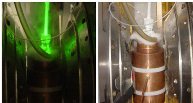
Figure 3: EPR tube is inserted in a resonator. An optical fiber is inserted in the EPR tube. It delivers 3mJ of green light to the sample inside the EPR tube. Also on a picture:
