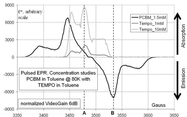
Figure 1: EPR measurements of TEMPO and PCBM at temperature of 80K and optimal concentration (~1mM).
