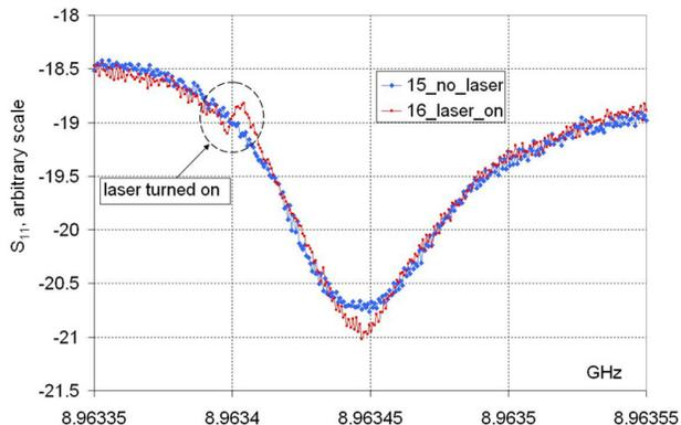
Figure 6: RF measurement of PCBM, 1mM. Magnetic field is at resonance, emission. Red points – laser on, blue points – laser off. We zoomed in on the resonance and observed a small change in coupling.
