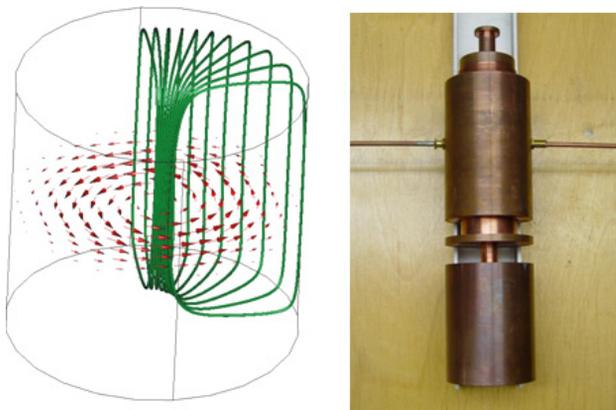
Figure 2:  $TE_{011}$  resonator fields: arrows – electric field, green – magnetic field lines. Photo of partially disassembled resonator showing tuning sections and RF connections.
