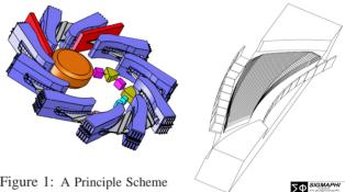
Figure 1: A Principle Scheme of the RACCAM Ring, a Variable Energy, Spiral Lattice Proton FFAG.
