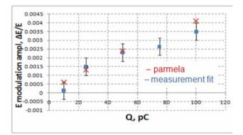
Figure 6: Measured (blue) and PARMELA simulated (red) energy modulation of 100fs, 10pC-100pC beam.
