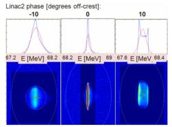
Figure 2: The scan of Linac2 phase. Lower plots are beam images on the BPM. Upper are energy projections (blue), and Gaussian fits (red).
