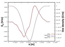
Figure 3: In a C-shaped compressor, the *z*-component of the electric field of a CSR-Wake and the corresponding 1D line density is shown.
